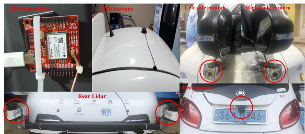
Figure 8. Multiple sensors (GPS, LIDAR, and camera) installed in the micro e-mobility vehicle.
